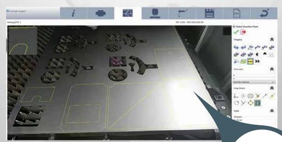
The program allows the user to add common cut, change cutting order, add / delete sheet framework cuttings, Add/delete lead-ins, microjoints, prepiercing, foil process.
