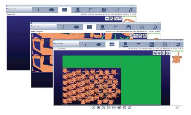
■ With Lantek Inside feature added to Aurora Plasma machines, you can make changes to userprepared programs, you can import dxf/dwg drawings or use the macro libraries. The program lets the user make a program directly from controller without computer need.
