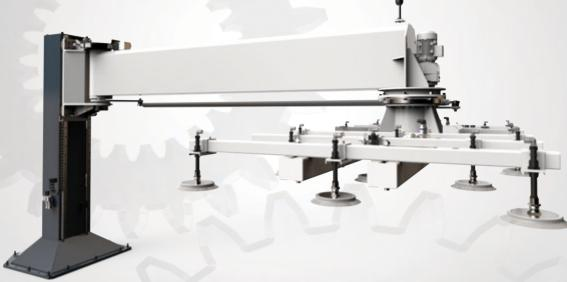
Lifting sytems can handle the sheet from floor level by vacuum pads. Rotation arm move the sheet on table. During this displacement; direction of the sheet not change and keep parallelism according to table.
