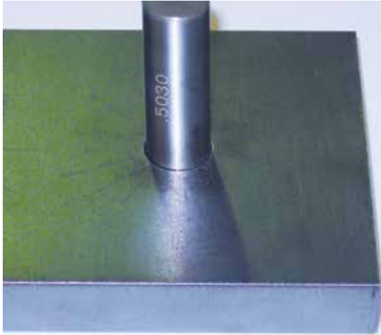
With True Hole technology cut with XPR Plasma
