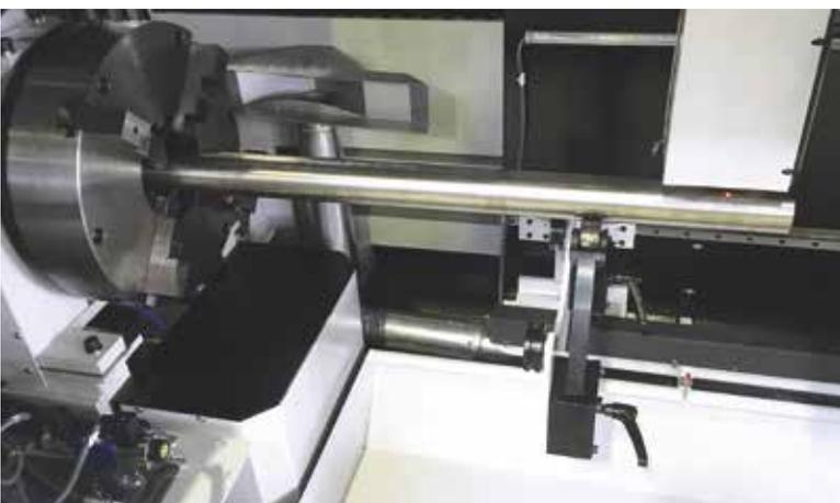
Pipe and tube profile rotation system
