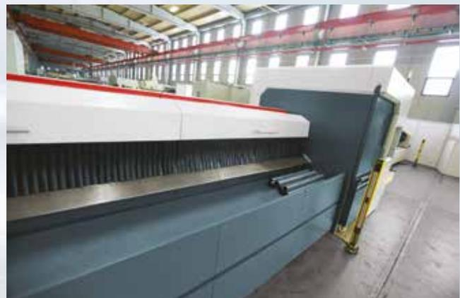
For longer parts than 800 mm, unloading table enters the cabin and unloads the parts.
