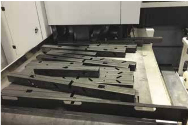
Tubes up to 6 m of lenght are removed by automatic unloading system with conveyor.
