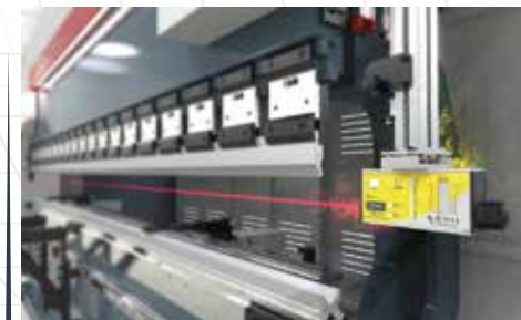
CE Laser Safety System
