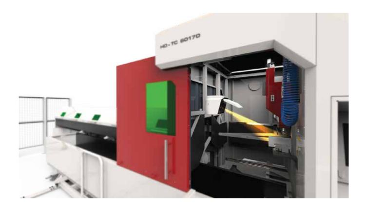
The Seam Detection sensor attached to the HD - TC machines detects the stitched surface when the pipe is loaded on the machine and provides the ability to rotate the operator's cut holes at any angle.
