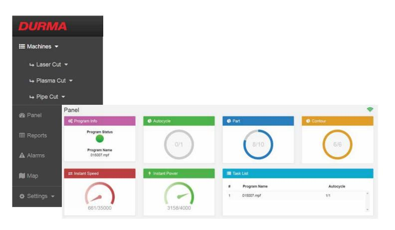
With the Cloud Option, which gives information about the old data, the users have more control over their machines by monitoring the machine from the desired environment and distance and monitoring the operating data of the machine.
