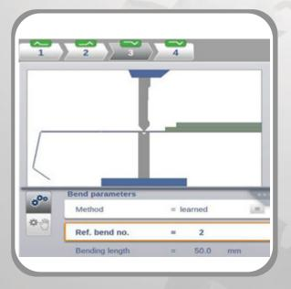
DAM system saves every bending step's springback distance. When you make a new bending on same sheet, system remembers that distance and uses it without making a measurement again. In this way, bending process will be faster and error range will be decreased.
