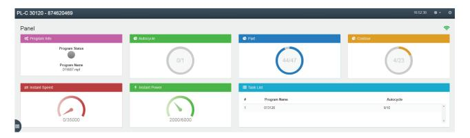
The user can follow the instant speed, parts / units and power information of the program cut on the machine via the panel. Other screens are the same as the clouds of laser machines.
